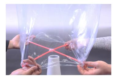
3. During the demonstration, have two students hold the bottom of the bag open as wide as possible. Set the blow-dryer to the hottest and highest settings. (If you have a very strong blow-dryer, you may want to set it to medium). Blow air into the bag, through the intersection of the straws, for about 3 minutes depending on the temperature of your classroom. Turn off the blow-dryer and then have students immediately let go of the bag.
