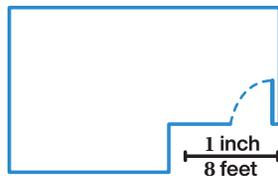
The scale of this floor plan tells us that 1 inch on the drawing represents 8 feet in the actual room.
